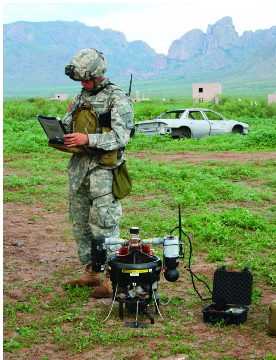
A soldier prepares a Micro Air Vehicle for flight at Fort Bliss, Texas
